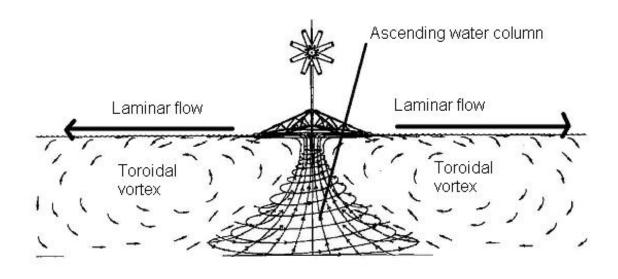
This toroidal vortex will only take place when having constant rotation of the impeller, meaning that local wind or solar conditions must be taken into account.
